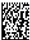
Figure E.3 – Example of GS1 DataMatrix symbol encoded with GTIN AI (01) and Lot Number AI (10).
