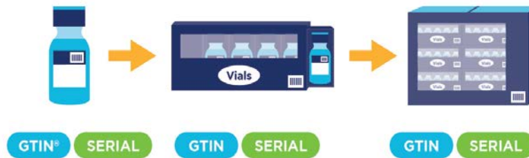
Figure 3-3 Example of packaging hierarchy in which all levels have been assigned both a GTIN and Serial Number
