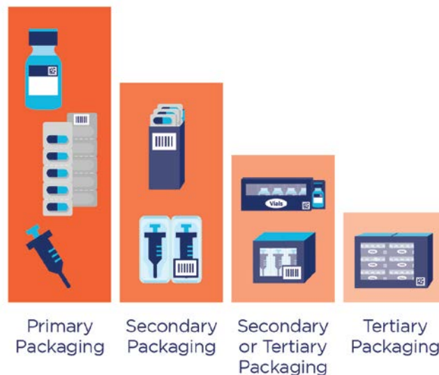
Figure 3-1 Examples of the packaging level hierarchies and the corresponding terminology for that level.
