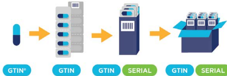
Figure 3-4 Example of a packaging hierarchy where all levels have been assigned a GTIN, but only some have been assigned a Serial Number.
