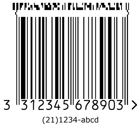
Figure 5.11.8-2. UPC-A symbol with a four-column CC-B component
