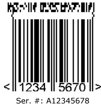
Figure 5.11.8-4. UPC-E symbol with a two-column CC-A
