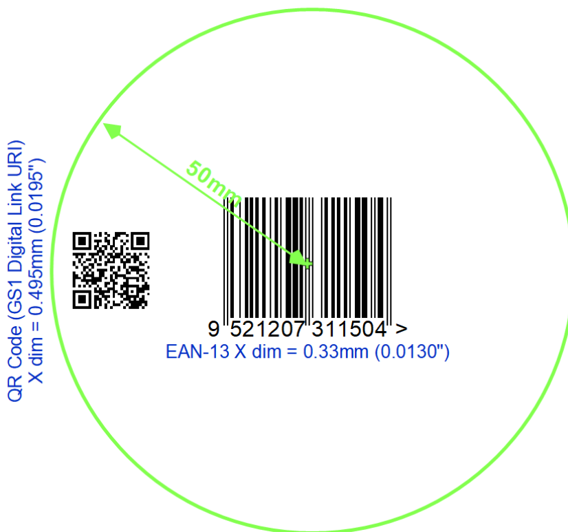
Figure 6.3.3.1-2. 2D barcode placement in relation to the linear barcode example
