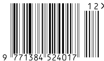
Figure 5.2.2.5.1-2. EAN-13 barcode with two-digit add-on symbol
