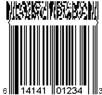
Figure 5.11.8-3. EAN-8 symbol with a three-column CC-A
