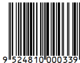
Figure 4.14-5. Example of EAN-13 with EAN/UPC HRI format
