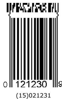
Figure 5.11.8-4. UPC-E symbol with a two-column CC-A
