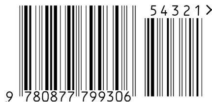
Figure 5.2.2.5.2-2. EAN-13 barcode with five-digit add-on symbol
