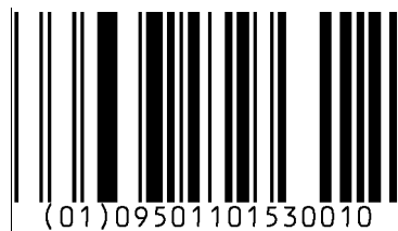
Figure 5.5.2.1.1-1. GS1 DataBar Omnidirectional barcode
