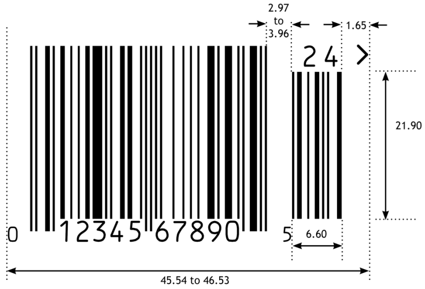
Figure 5.2.6.6-5. UPC-A barcode with two-digit add-on symbol
