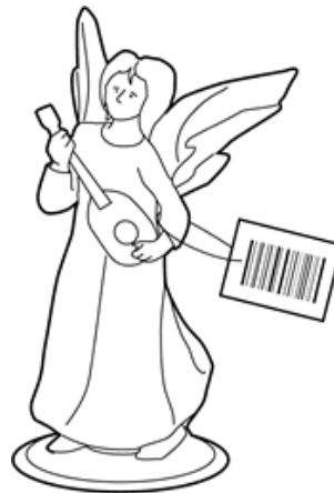
Figure 6.4.16-6. Tableware using spot label below backstamp
