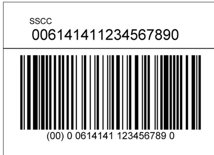
Figure 6.6.5-1. The basic label: an SSCC
