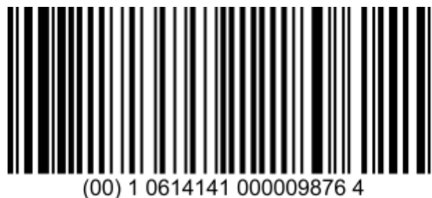
Figure 2-1 GS1-128 barcode containing SSCC
