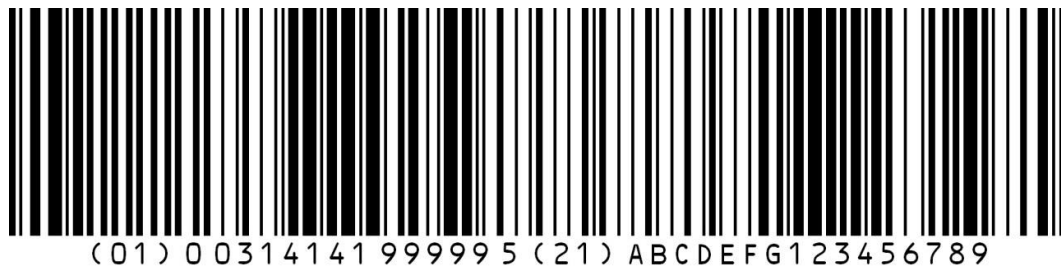
Figure 5-5 GTIN with Serial Number Encoded in a GS1-128
