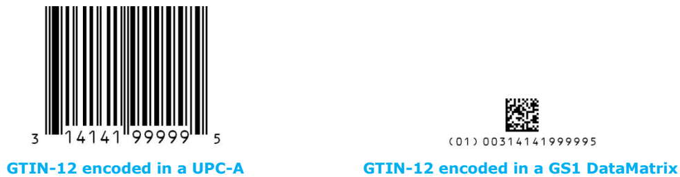
Figure 5-1 GTIN-12 in a UPC-A and GS1 DataMatrix
