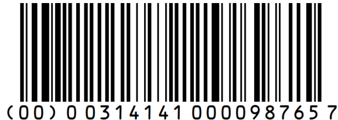
Figure 5-2 SSCC Encoded in a GS1-128
