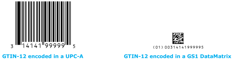
Figure 5-1 GTIN-12 in a UPC-A and GS1 DataMatrix
