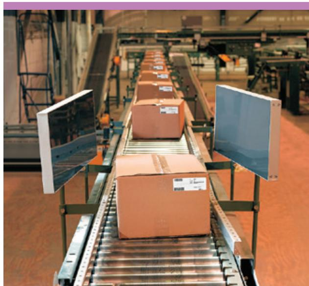
**Case-level scanning at a brand owner's distribution center via a conveyor RFID tunnel.**
