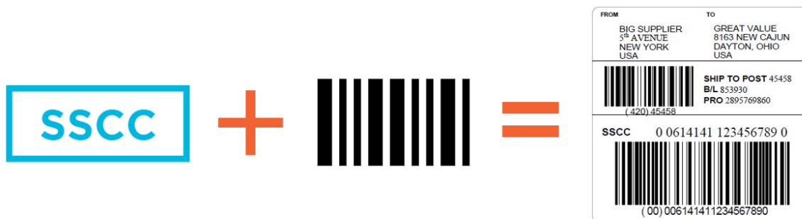
Figure 5-3 Example of an SSCC encoded into GS1-128 on a Logistic Label
